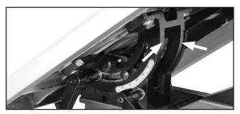
Figure 15. Trunnion lubrication location.
